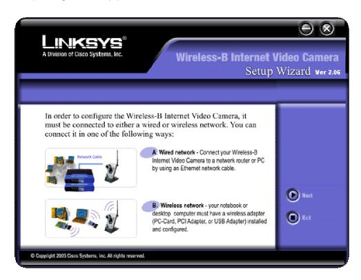
4. Make sure the Camera is correctly connected to your network and Click Next
